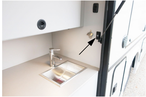
Tailgate Sink Drain Pump Switch (Located near exterior (tailgate) sink) -Typical View
