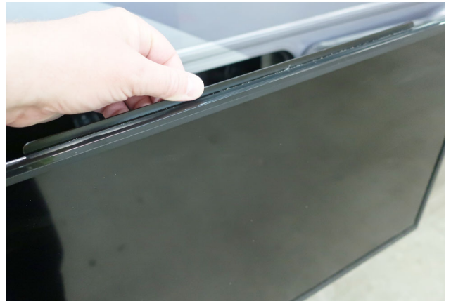
When folding the TV back down press on the metal bracket above- DO NOT press on the screen as damage may occur. -Typical View
