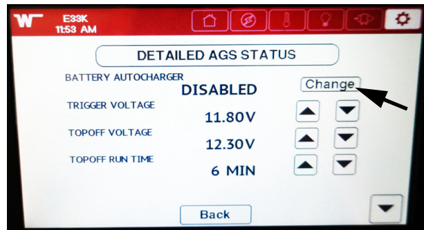
Detailed AGS Status page with Battery Autocharger selection. -Typical View
