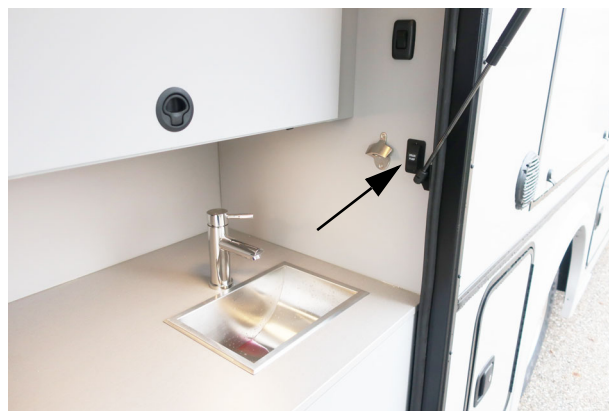
Sink Drain Pump Switch (Located near exterior sink) -Typical View
