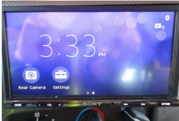
Swipe to the right to access the second page of the main menu containing the rear camera and settings functions. -Typical View
