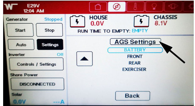
Selecting the down arrow again will take you to screen 3 which has the AGS (Auto Start Generator) Settings. -Typical View
