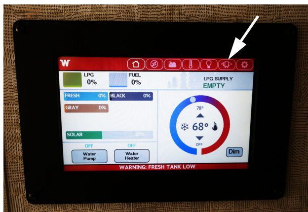
From the home screen on the monitor panel, select the slideout/awning icon. -Typical View
