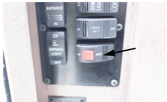
Entry Step Switch Located near entrance door (The switch configuration may vary) -Typical View
