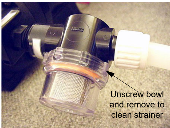
Water Pump Strainer -Typical View
