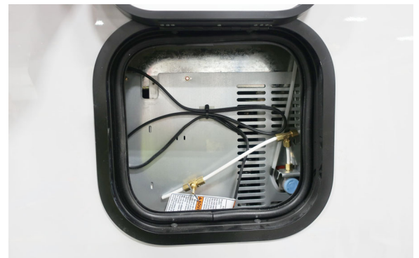
Refrigerator Access Door (open) -Typical View
